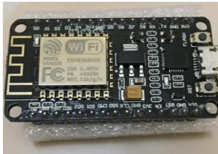
**Gambar 2.3** NodeMCU
