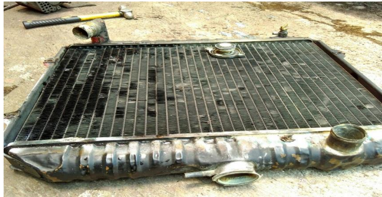
Gambar 4.3 kondisi Radiator Lancer SL
