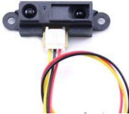
Gambar 2.3 Sensor SHARP GP2Y0A21 (sumber. http://www.conrad.com/ce/en/product/185350/Sharp-GP2Y0D02YK-Distance-Sensor-GP-2-YOD-02-YK-5-Vdc )
