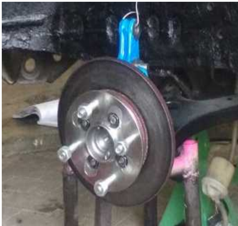
Gambar 4.24 Stering knuckle arm baru
