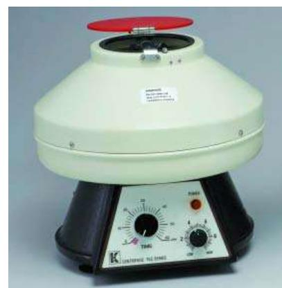
Gambar 2. 1 Alat centrifuge [3]
