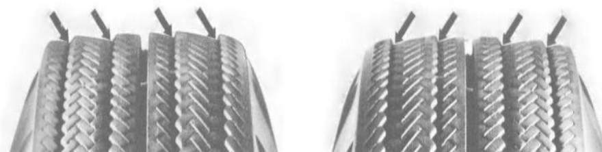
Gambar 2.36 Keausan Ban Akibat Toe – out .
