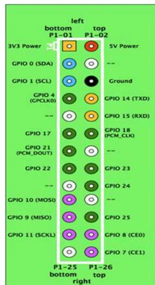
Gambar 2.11 Pin GPIO *Raspberry Pi*
