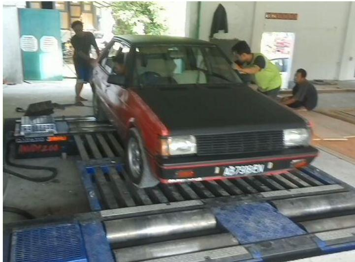
Gambar 3.9. Alat Dyno Test Mobil
