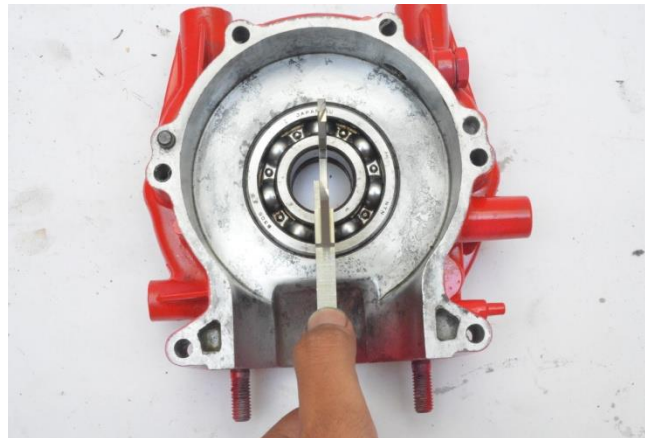
Gambar 4.8 Pengukuran bearing as depan ATV Toyoco G16ADP 2 Tak
