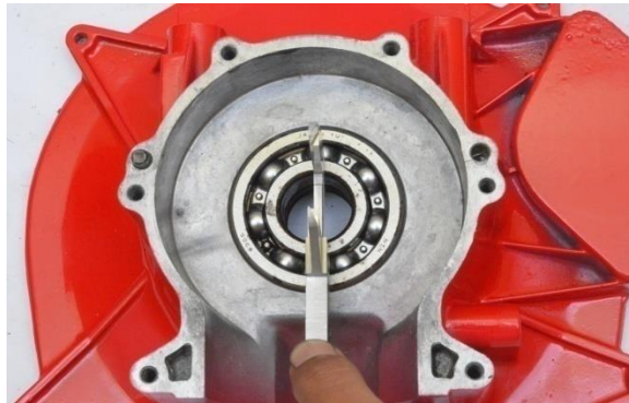
Gambar 4.7 Pengukuran bearing as belakang ATV Toyoco G16ADP 2 Tak
