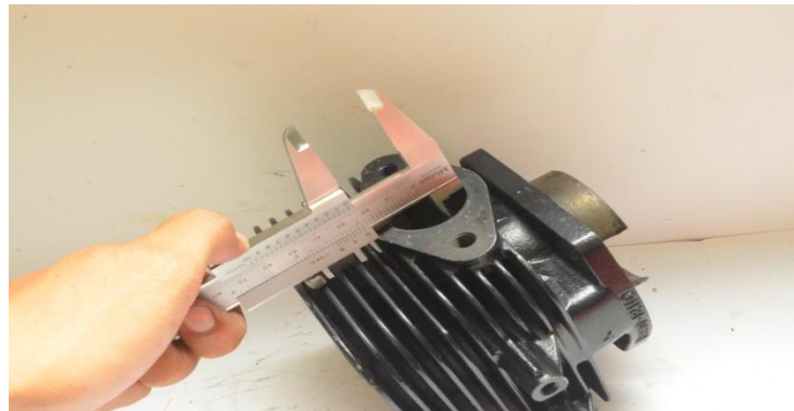
Gambar 4.16 Pengukuran lubang ex-haust ATV Toyoco G16ADP 2 Tak
