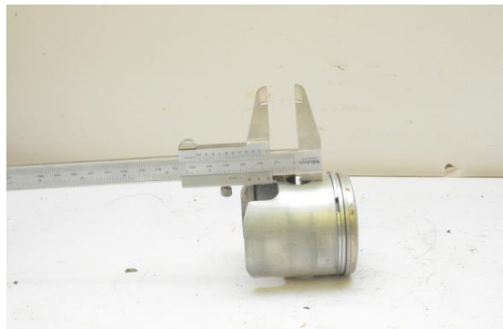
Gambar 4.6 Pengukuran lubang pen piston ATV Toyoco G16ADP 2 Tak
