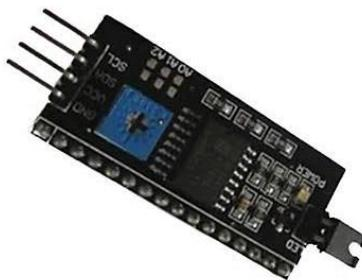
**Gambar 2.9** LCD Modul I2C
