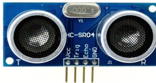
Gambar. 2.4. Modul sensor ultrasonic HC-SR04
