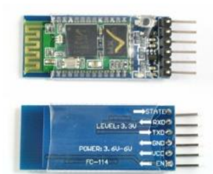
Gambar 2.4 Modul Bluetooth HC-05
