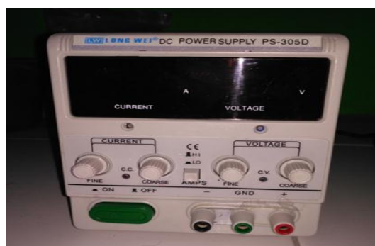
Gambar 3.2 DC Power Supply
