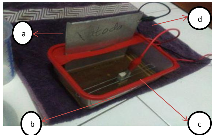
Gambar 3.23 Proses Anodic Oxidation. (a) Katoda, (b) Spesimen/Anoda, (c) Positif Power Supply, (d) Negatif Power Suply
