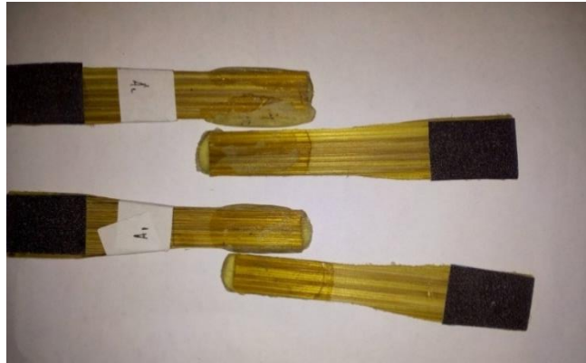
Gambar 4.7 Sambungan Lap Joint Tanpa Strap
