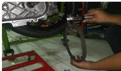
Gambar 3.11 Proses mengukur drive belt
