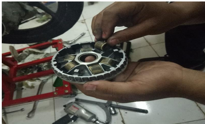
Gambar 3.24 Proses memasang weight roller
