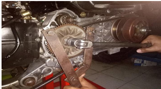
Gambar 3.4 Proses melepas drive pulley face
