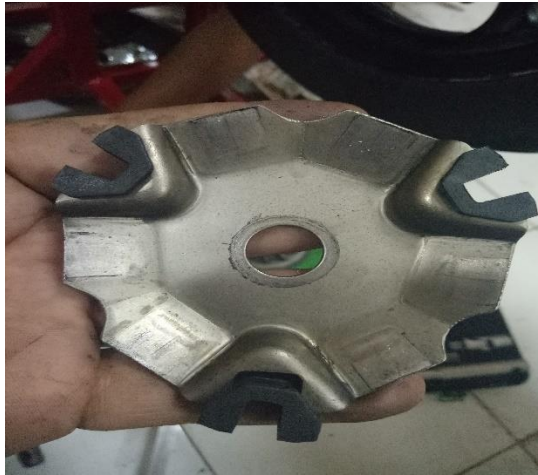
Gambar 3.14 Proses memeriksa ramp plate
