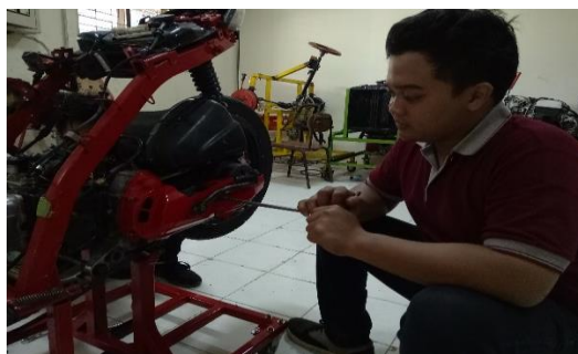
Gambar 3.3 Proses melepas cover CVT
