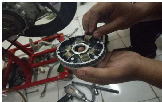
Gambar 3.8 Proses melepas weight roller
