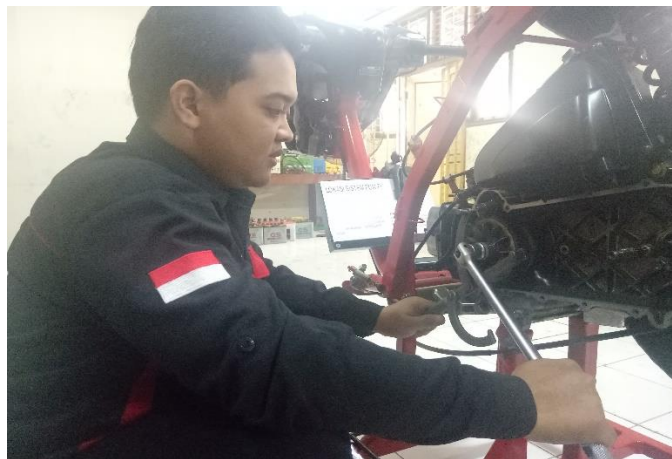
Gambar 3.28 Proses memasang drive pulley face
