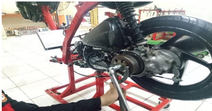
Gambar 3.9 Proses melepas drive belt
