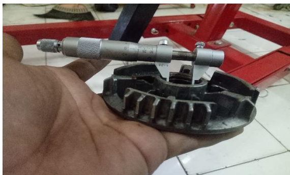
Gambar 3.13 Proses mengukur movable drive face
