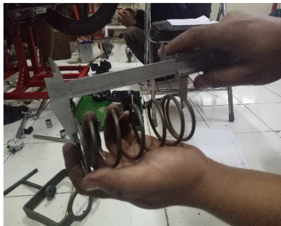
Gambar 3.17 Proses mengukur pegas driven face
