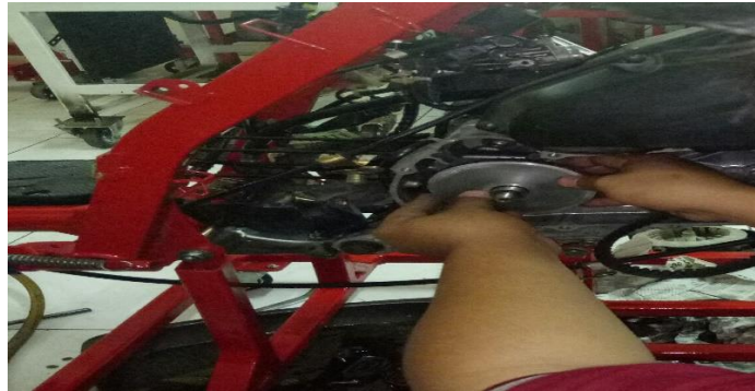
Gambar 3.27 Proses memasang boss movable drive face
