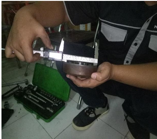
Gambar 3.16 Proses mengukur outer clutch
