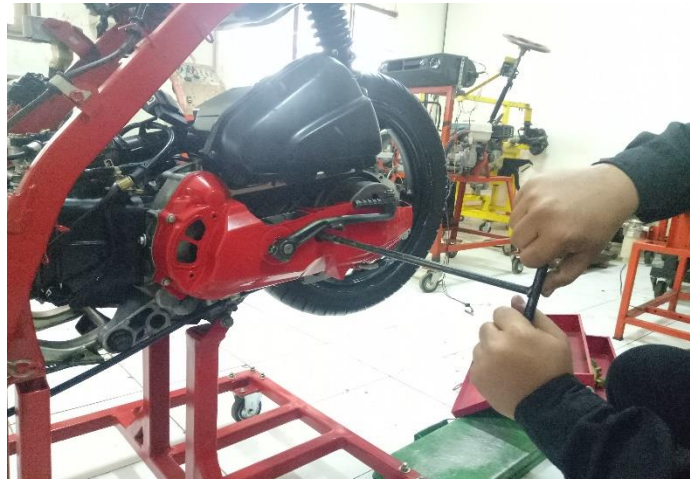
Gambar 3.30 Proses memasang cover CVT
