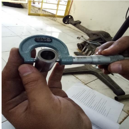
Gambar 3.12 Proses mengukur boss movable drive face
