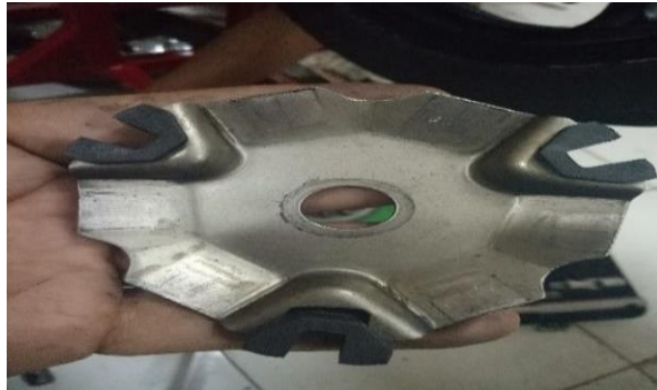
Gambar 3.7 Proses melepas slide piece
