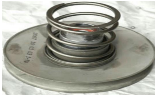
Gambar 3.22 Proses memasang driven face
