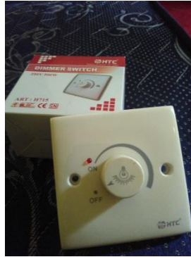
Gambar 3.2 Dimmer SCR ( Speed Controller Regulator)
