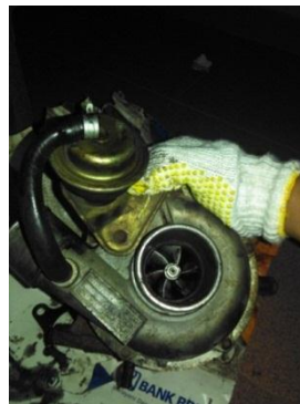
Gambar 3. 6 Turbocharger KIA Carnival 2.9 Diesel Type IHI RHF5
