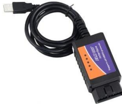
Gambar 3.1 Scanner Code Reader ELM 327
