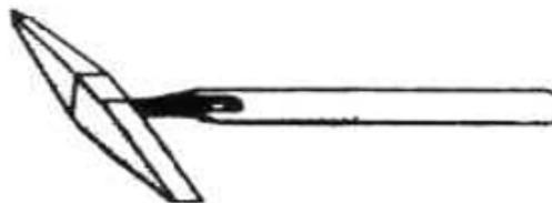
Gambar 3.2 Palu Las (*chipping hammer*)
