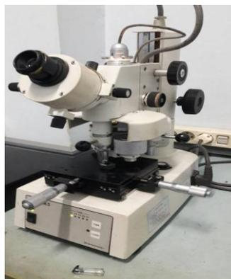
Gambar 2.14 *Micro hardness tester*
