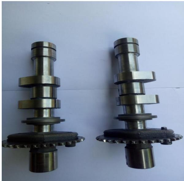
Gambar 2.4 Chamshaft Camshaft Suzuki Satria F 150cc
