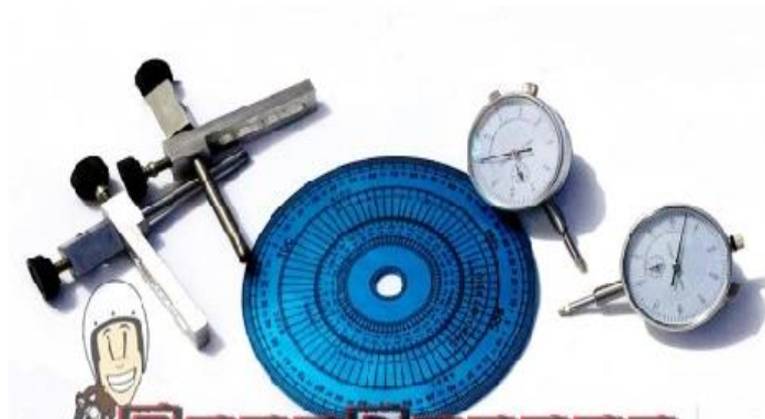
Gambar 3.10 Alat ukur durasi Camshaft ( http://www.tanzracing.com )
