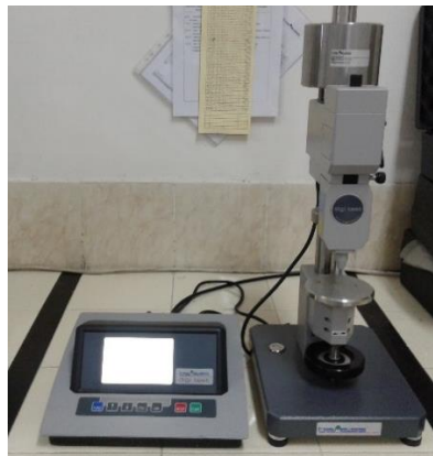
Gambar 3.5 Alat uji kekerasan Shore D (BBKKP Yogyakarta, 2017)
