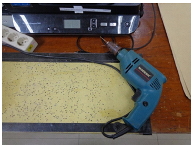
Figure 5. Drill Used to perforate the edges of the book to ease the bindery.
